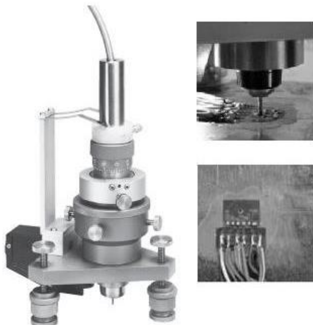
Figure 4.4. Vishay RS 200 Milling Guide (drilling tool) existing at GTR lab and experimental procedure.
