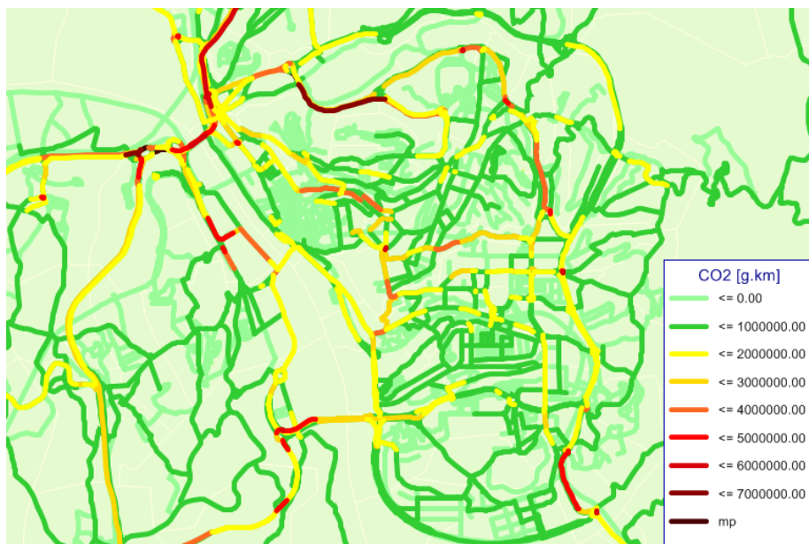
Figure 22 – CO 2 emission road assignment for the city of Coimbra – road tolling policy
