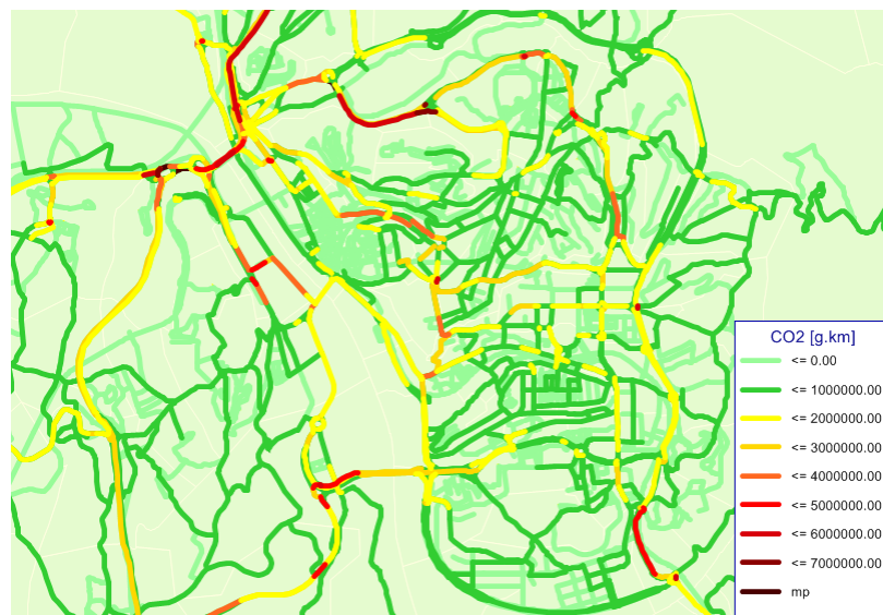
Figure 24 – CO 2 emission road assignment for the city of Coimbra – complex TDM policy
