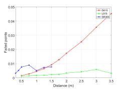
Figure 5: Point-to-plane RMSE D415 vs L515 vs SR305 -  $\pm 10$  cm.
