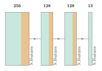
Figure 4.9: 6DoF pose estimation network. Light green rectangles are MLP's. Dark yellow bands represent ReLU activation.
