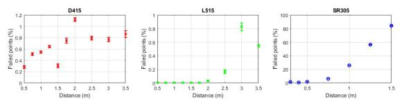
Figure 3.3: Failed Points - D415 vs L515 vs SR305.
