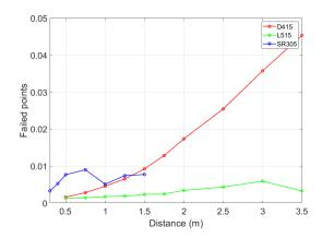
Figure 3.6: Point-to-plane RMSE D415 vs L515 vs SR305 -  $\pm 10cm$ .
