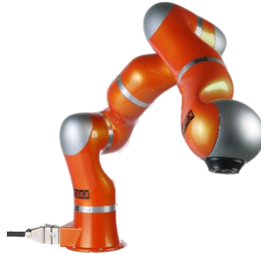
Figure 2.1. KUKA® LWR, the first commercialized version of the lightweight robot co-developed with DLR .
