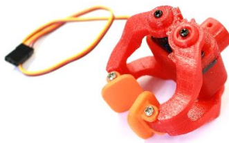
Figure 6.2. Glimpse of the developed gripper.
