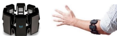
Figure 7.4. Myo™, a gesture control armband developed by Thalmic Labs™.
