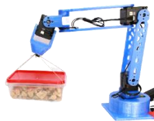
Figure 7.3. The robot handling a 400 g load.
