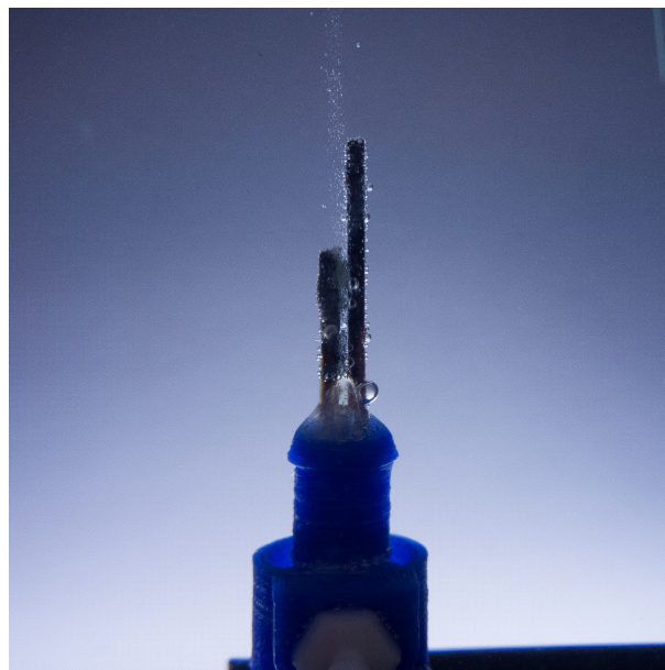
Figure 9.6: Water electrolysis occurring in the actuator's end terminal connected to a 16 V (DC) power supply.
