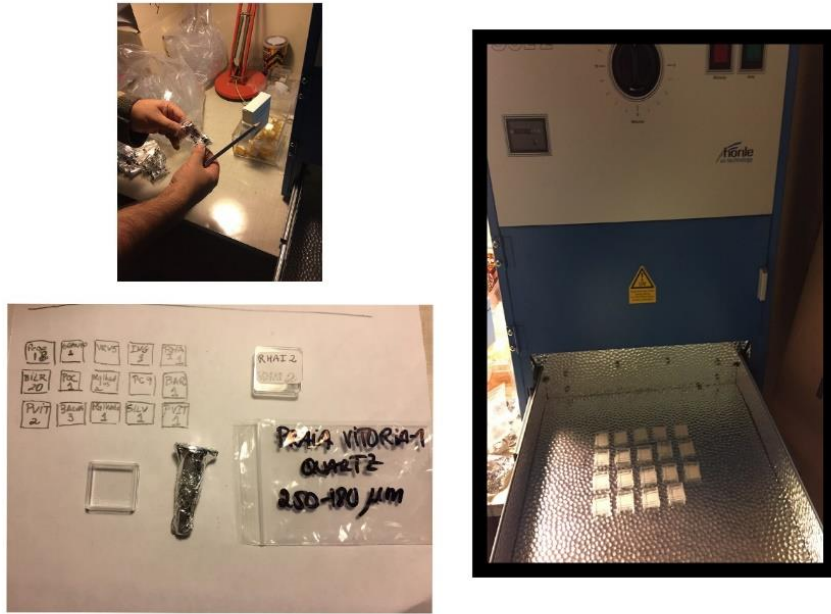
Figure II. 26. The Dr Honhle SOL2 solar simulator equipment, scheme of each sample location and sample preparation.
