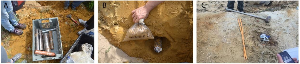
Figure II. 19. Material and methods used in the fieldwork. A, B- PVC or metal tubes, ziplock bag (C) metal cap, hammer and hand trowel, measuring tape, portable GPS.
