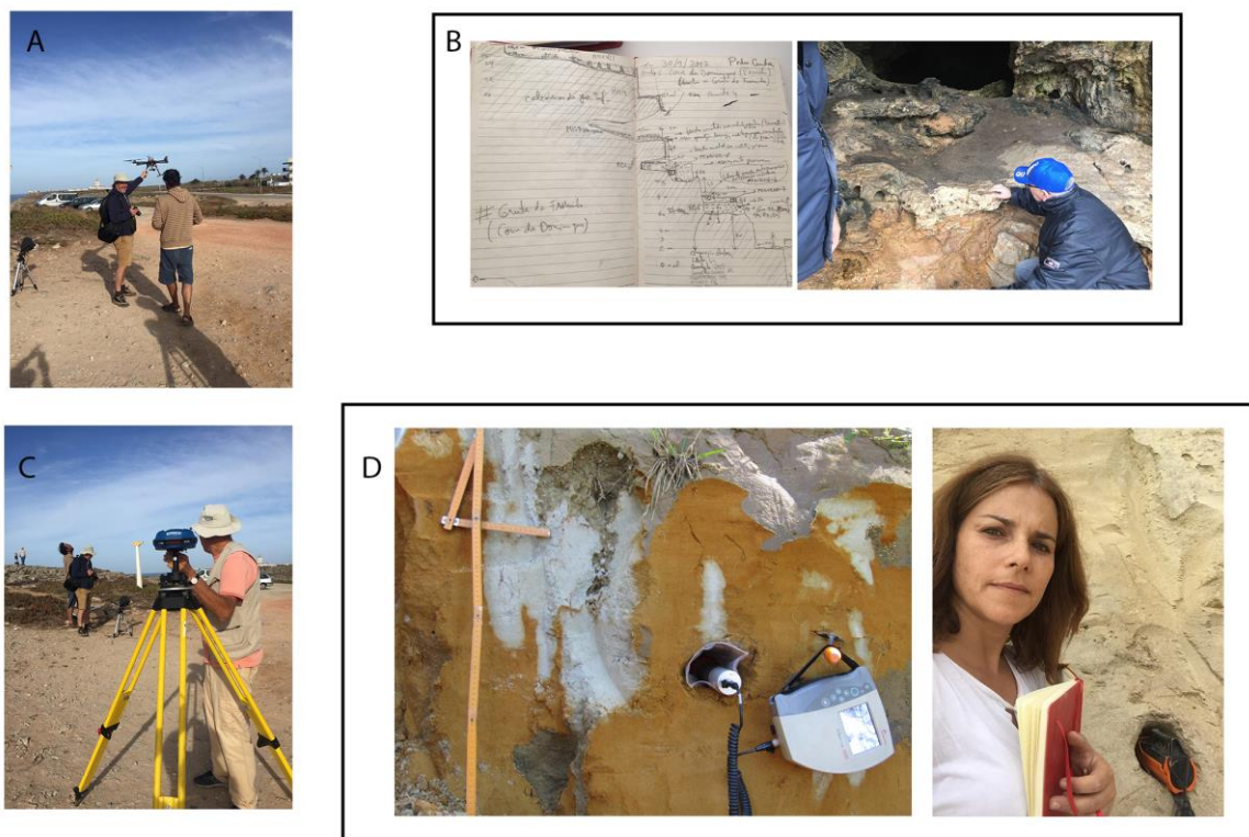
Figure II. 20. Material and methods used in the fieldwork. A-photo camera et A - aerial vehicle (UAV); B.;C- GPS-RTK; D-portable spectrometers gamma-ray (Nal probe connected to an Inspector 1000 (Canberra) and RS230).
