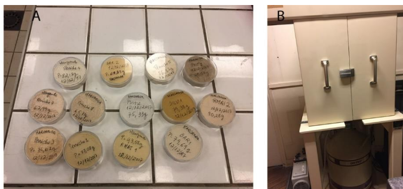
Figure II. 27. A - Samples weighed and labelled for the gamma-ray spectrometry measurements; (B) - gamma spectrometer.
