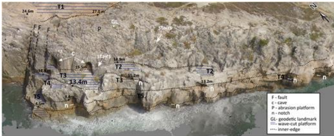
Figure IV. 8. Three-dimensional model, with high-resolution (3D model with the texture of the photographs and resolution of 4.6 cm/pix and a high precision Digital Surface Model (MDS) with a resolution of 9, 2 cm/pixel) of the coastal terrace staircase at Furninha Cave site, located at ~850 m SE of the Carvoeiro Cape. The several marine terraces (Tm1 to Tm6) and other geomorphological elements are indicated.
