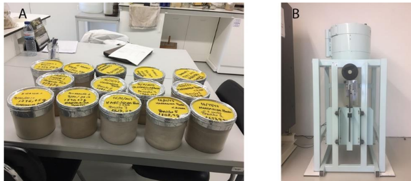
Figure II. 28. A. - Marinelli type beakers filled with each sample. B - high-resolution gamma-ray spectrometer of Radioactivity Laboratory (University of Coimbra).
