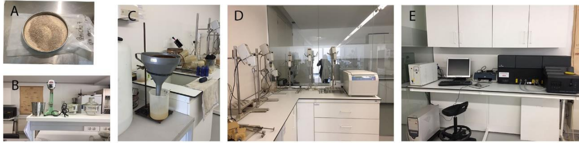
Figure II. 21. Methodologies used in sedimentological and textural analyses A. sample for granulometric analysis in an analytical sieve; B- Stirrer equipment; C-63 µm mesh sieve to separate the fine fraction from coarser ones; D- centrifuge; E-Beckman Coulter laser granulometer.
