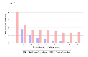
Fig. 5. Disconnection per controller number – disjoint paths versus separate controllers – Polska average
