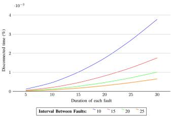
Fig. 7. Reliability vs Failure Duration and Frequency - Germany50 average
