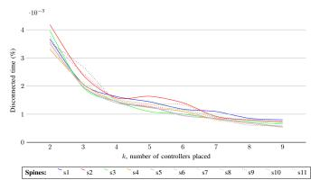
Fig. 6. Reliability when using different spines – Germany50 average, k=2 to 9
