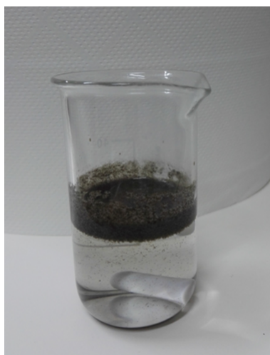
Figure B1: Photograph of phase separation when CTAB was added into the solution containing ethanol-water as solvent and graphene oxide.
