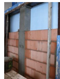
Figure 2.74 – GHB: wall specimen being assembled in the frame [210].
