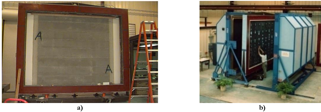
Figure 2.62 – ORNL facility: a) unfinished Rastra wall on the hot box test support frame [189]; b) GHB [158].
