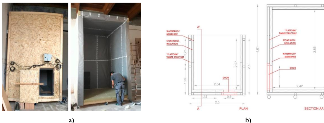
Figure 2.90 – In situ hot box: a) apparatus; b) drawing of the metering box horizontal plan and vertical section [235].
