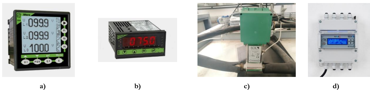
Figure 4.15 – Electric analysers: a) triphasic Sfero model Diva 11 [285]; b) Sfero model Diva 5 [286]; c) Electromagnetic flowmeter; and d) Heat meter integrator.
