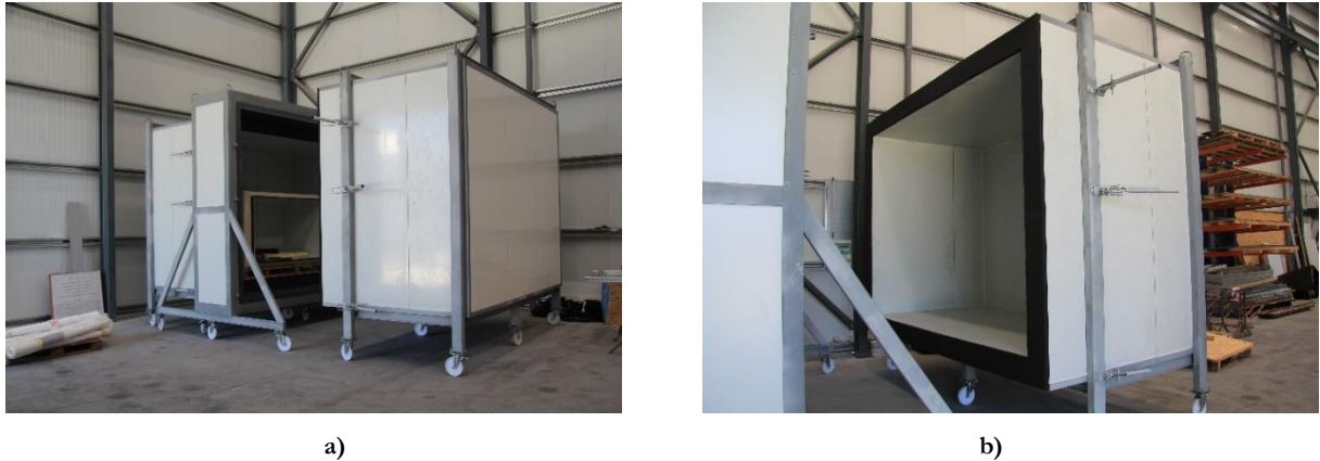
Figure 4.7 – HB apparatus passive components after assembly.
