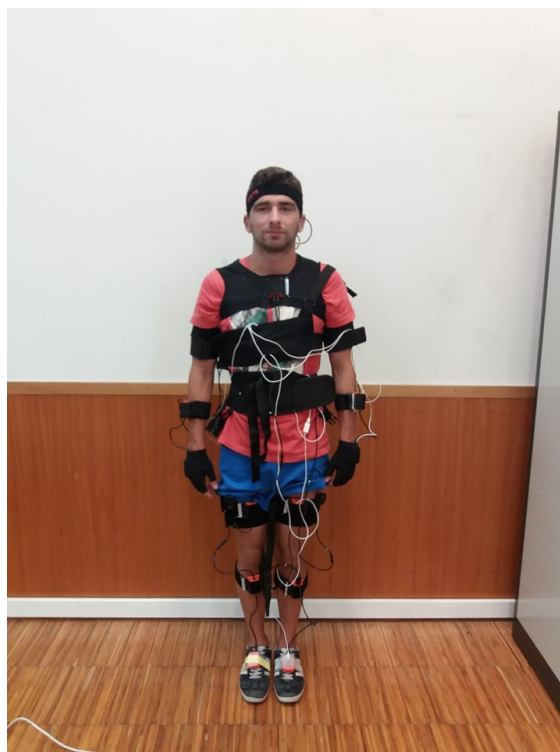
Figure 4.6: Xsens MVN inertial motion capture suit consisting of 17 inertial and magnetic sensor modules. A calibration procedure is required to determine sensor to body alignment and body dimensions.
