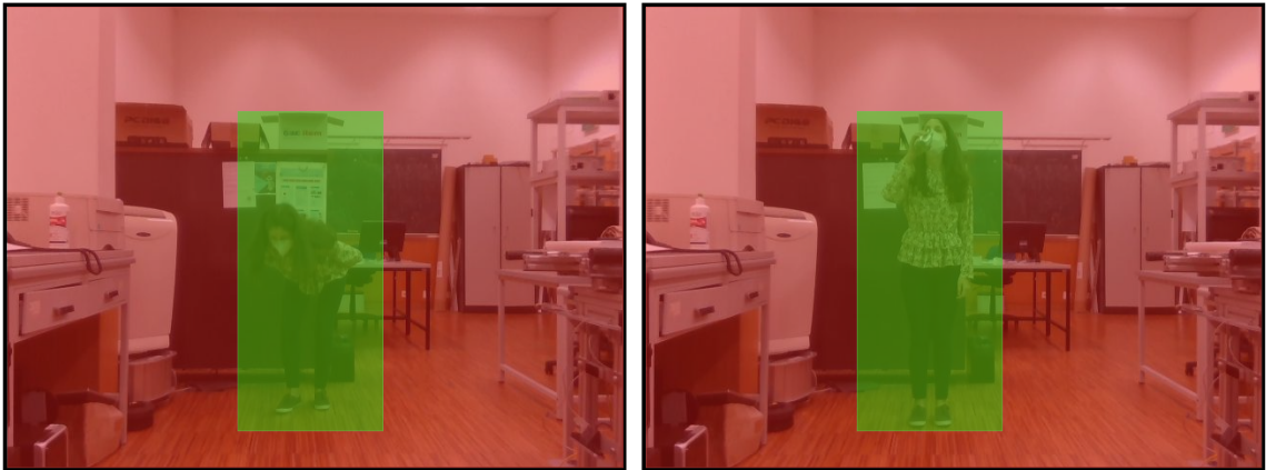
Figure 5.3: Comparison between two frames depicting different activities, drinking water and vomiting. It shows a red region, which is common to both pictures, that does not contribute with any relevant information to distinguish between the two activities. The green region contains the area where the activity is being performed.
