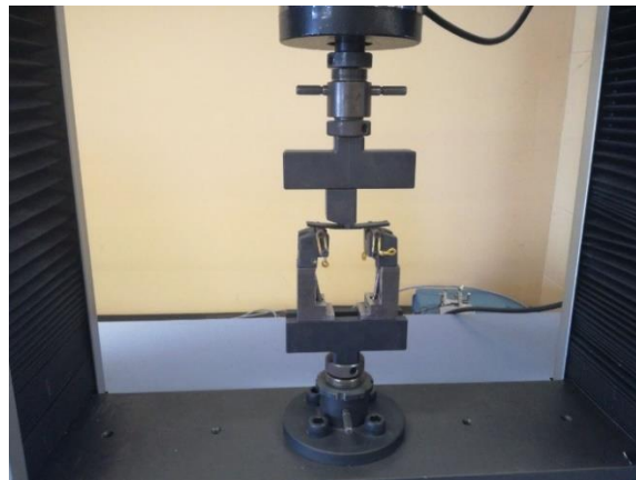
Figure 7: Shimadzu Autograph AGS-X during three-point flexural test.
