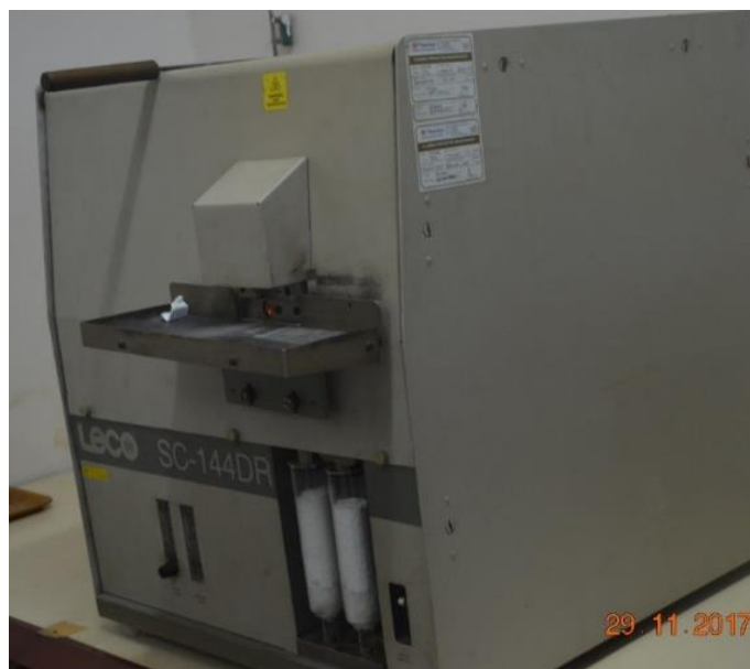
Figure 3.6 -The LECO SC-144DR equipment for analysis of TOC.
