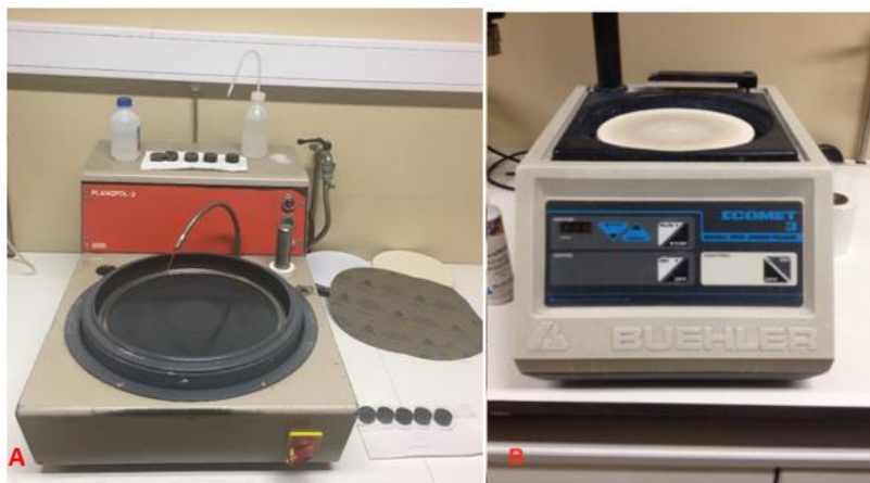
Figure 3.4 - [A] Pre-polishing equipment. [B] Final polishing equipment.
