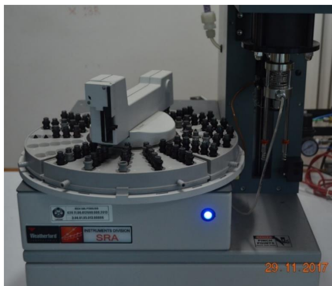
Figure 3.7 - Source Rock Analyser equipment.
