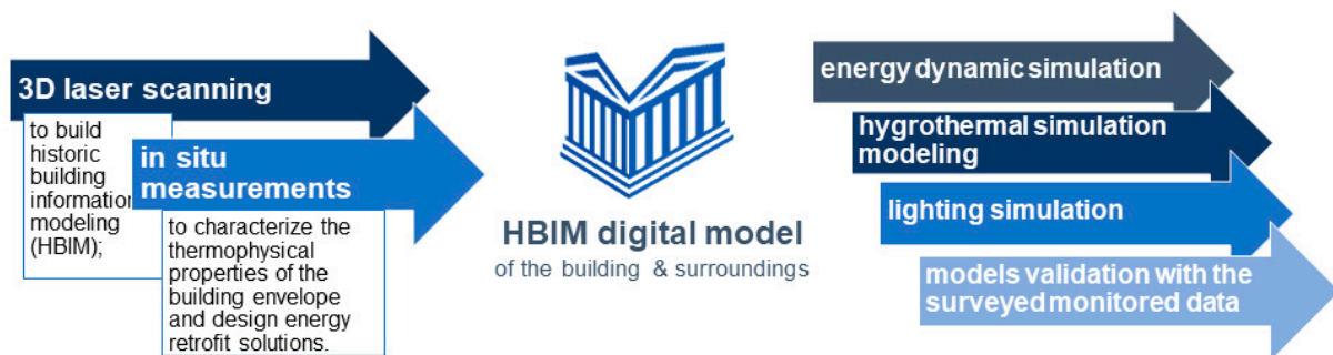
Figure 5. Historic building information modeling (HBIM) digital model premises and outputs.
