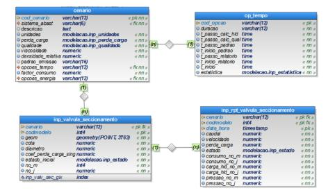
**Figure 3.** Attributes and domains considered in order to characterize the desired scenario and to specify temporal options, exemplifying relationships established for the association of results with the scenario and respective modelled components (valve particular case).
