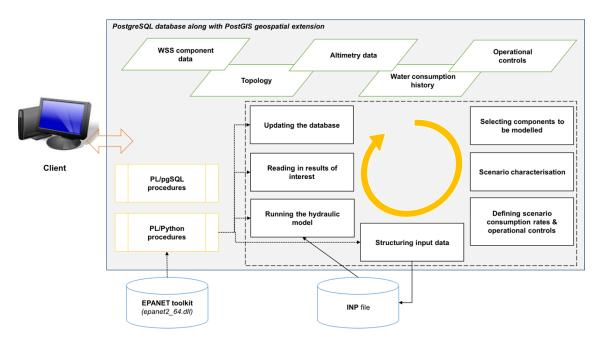
**Figure 2.** Conceptual model of the system proposed: data stored in the system and functions implemented on the geospatial database management system (DBMS) enable the construction of the hydraulic model (based on EPANET numerical model) and running it (through SQL instructions).
