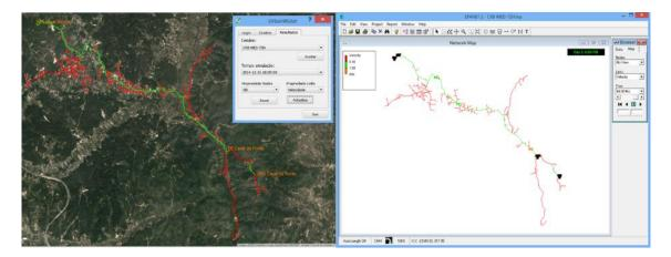
**Figure 11.** Visual representation of velocity, in Quantum geographical information system (QGIS) and EPANET, respectively.
