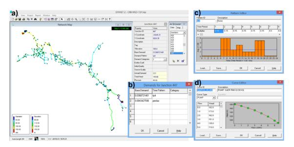
**Figure 9.** Visualization on EPANET of information contained within the INP file created: (**a**) geospatial representation of Casal-do-Ribeiro WSS; (**b**) customer consumption at junction node 447; (**c**) consumption rate; (**d**) pump characteristic curve at Casal-da-Fonte pumping station.
