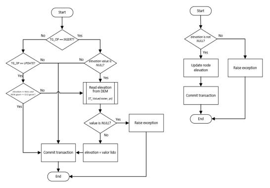
Figure 5. Flowchart of elevation\_insert and elevation\_updt trigger procedures.
