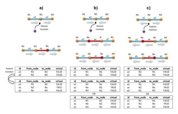
**Figure 4.** Representation of the arc-node topological model and its update after the insertion in the system of a specified component: (**a**) same direction of flow at the insertion point; (**b**) converging flow directions at the insertion point; (**c**) diverging flow directions at the insertion point.
