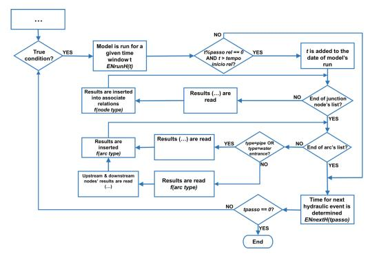
Figure 7. Partial flowchart of processa\_inp procedure, which runs the hydraulic modelling process.
