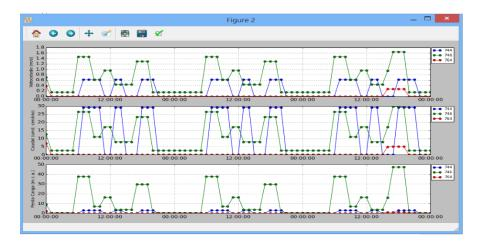
**Figure 10.** Velocity (m/s), flow (m<sup>3</sup>/h) and head loss (m/km) for 744, 746, and 764 pipes, over the simulation period (*UrbanWater* plugin).
