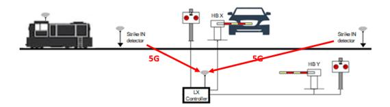
Figure 1.2: Railway Signalling scenario [47]
