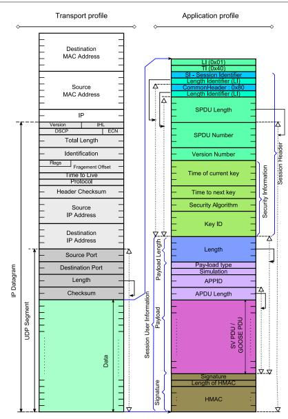
Figure 3.3: R-GOOSE PDU [22]
