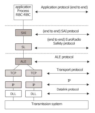
Figure 3.2: UNISIG Subset-098 Protocol Stack [56]
