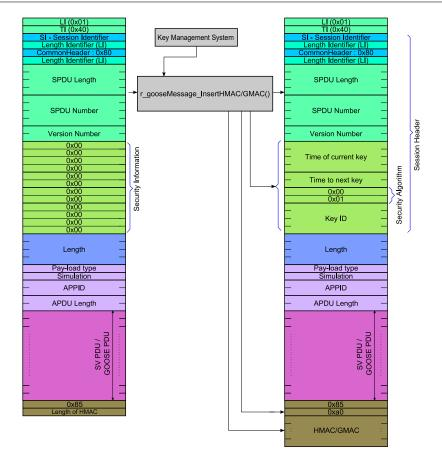
Figure 4.3: Diagram of InsertHMAC/GMAC funtions
