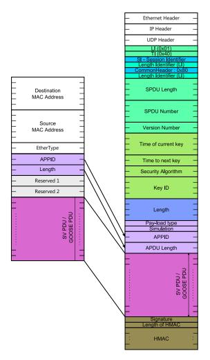
Figure 4.1: Conversion from GOOSE to R-GOOSE
