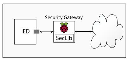
Figure 4.2: Diagram of proposed Security Gateway
