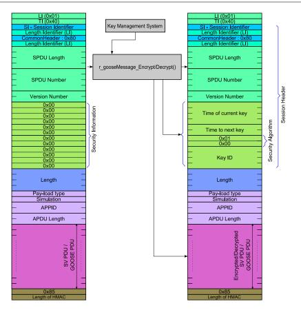
Figure 4.4: Diagram of Encrypt/Decrypt funtions
