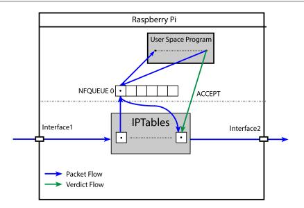
Figure 4.5: Bridge Diagram - Interaction between IPTables, Netfilter NFQUEUEs and user space program in a one way communication
