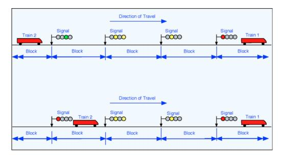
Figure 2.1: Railway signalling operating on segments context [57]
