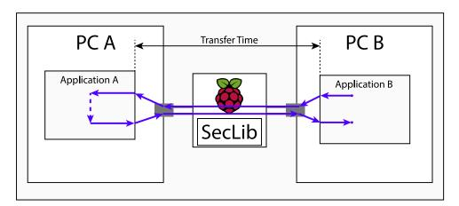
Figure 5.16: Diagram of Ping testing and relation with Transfer Time
