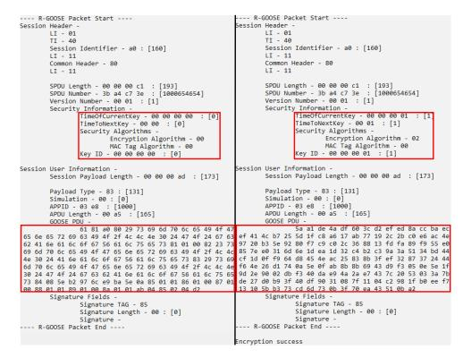
Figure 5.6: Encryption of an R-GOOSE packet
