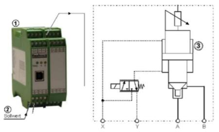
Figure 2.4 – Schematics of the RE4 controller, Hauhinco manual
