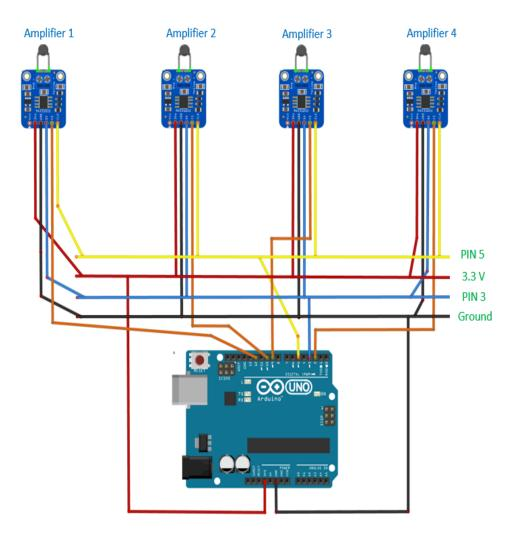
Figure 2.12 – Detail of the wiring scheme between the Arduino<sup>®</sup> and the four thermocouple amplifiers.
