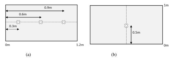
Figure 4.2 – Thermocouples distribution in (a) front of the barrier (b) back of the barrier
