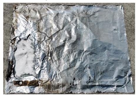
Figure 4.6 – The fire barrier fabric after the first experiment
