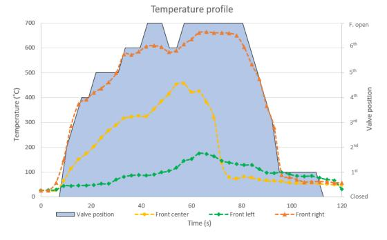
Figure 4.8 – Fabric temperature profile in the second test
