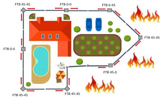
Figure 1.5 – Example of fire-proof barrier layout along with a dwelling, (Costa, 2018)
