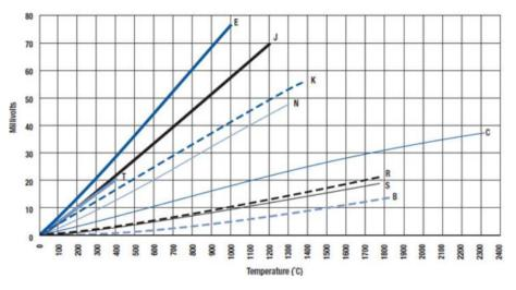
Figure 2.10 - Response of the different types of thermocouples
