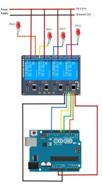
**Figure 2.8** – Scheme of the connection between Arduino<sup>®</sup> and controller via relays The relay module complete specifications sheet is available in ANNEX A.
