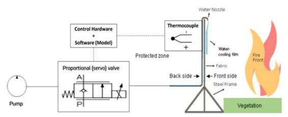
Figure 2.1 - Barrier with water distribution control system, (Viegas, et al., 2019)
