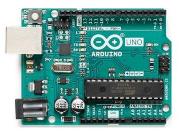
Figure 2.6 – Arduino® Uno Rev 3 board
