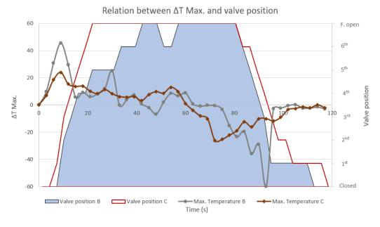
Figure 4.15 – Maximum temperature with valve position
