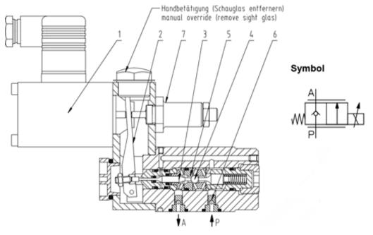
Figure 2.3 – Valve operating scheme
