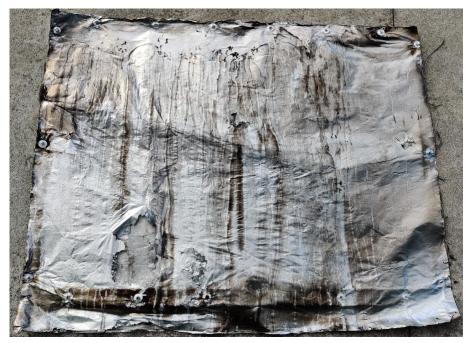
Figure 4.13 – The fire barrier fabric after the first experiment
