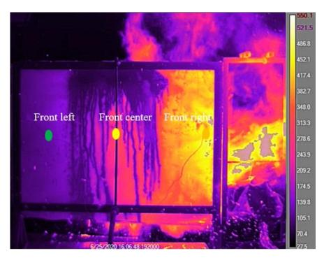
Figure 4.9 – Fabric temperature distribution at t=66s during the second experiment
