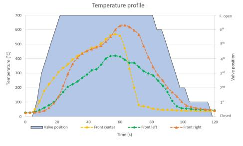
Figure 4.11 – Fabric temperature profile in the third test
