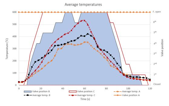
Figure 4.14 – Average temperature and valve position for each test
