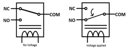
Figure 2.7 – Representative scheme of the relay operation
