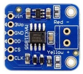
Figure 2.11 – The thermocouple amplifier MAX 31855 used
