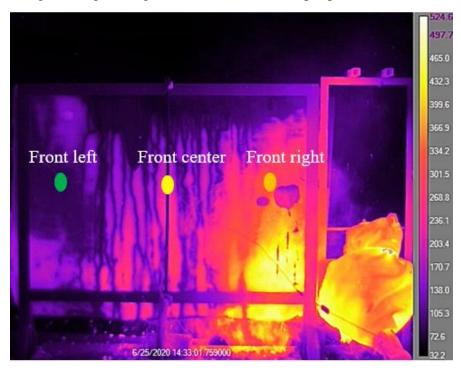
Figure 4.7 – Fabric temperature distribution at t=75s during the first experiment
