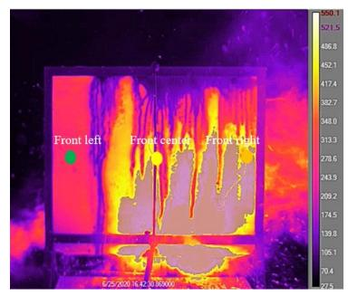
Figure 4.12 – Fabric temperature distribution at t=66s during the third experiment
