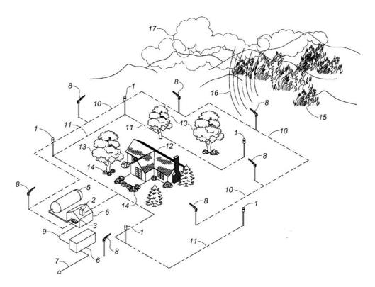
Figure 1.3 – Possible format for positioning the components of the WSS
