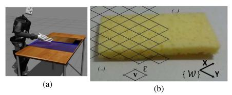
**Fig. 1.** a) Results from a previous work [3], demonstrating a haptic discontinuity following task: straight line geometry. In this work, the haptic exploration tasks are more challenging: three materials and discontinuities with other geometries than straight lines. b) Illustration of a 2D isometric grid partitioning a real world workspace area. Each cell v has a dimension  $\varepsilon$  and is described by position (*x*,*y*) expressed in {*W*}.
