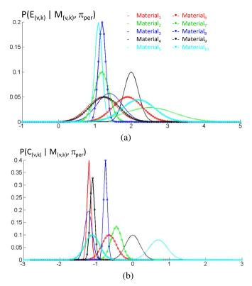
**Fig. 5.** Representation of  $P(E_{(vi,k)}|M_{(vi,k)}, \pi_{per})$  (a)) and  $P(C_{(vi,k)}|M_{(vi,k)}, \pi_{per})$  (b)) learned for 10 reference materials. Data extracted from [10].
