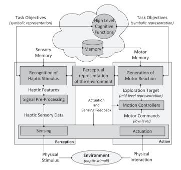
Fig. 2. Conceptual representation of the action-perception loop [7] involved in the haptic exploration of surfaces [8]. In this work, the objectives of the task and corresponding solution is represented in two levels: symbolic and mid-level.
