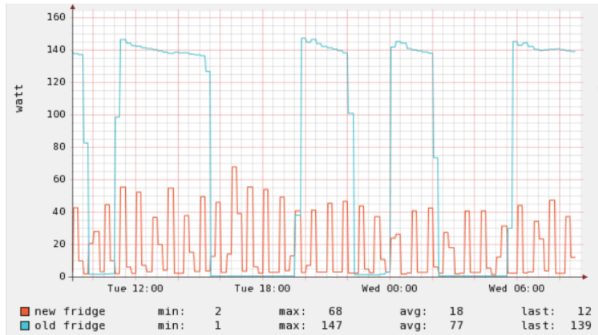
Figure 2.4: Power consumption of a new vs. old fridge.(From [6])
