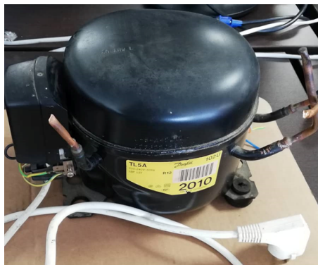
Figure 5.3: TL5A Danfoss Compressor from a freezer.
