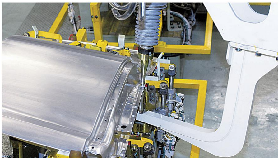
Figure 2.3 FSSW industrial application in Mazda Motor Corp.[14].
