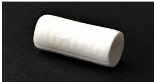
Figure A.1: Picture of a sample of an aerogel, obtained by Agostinho (2019) [60].
