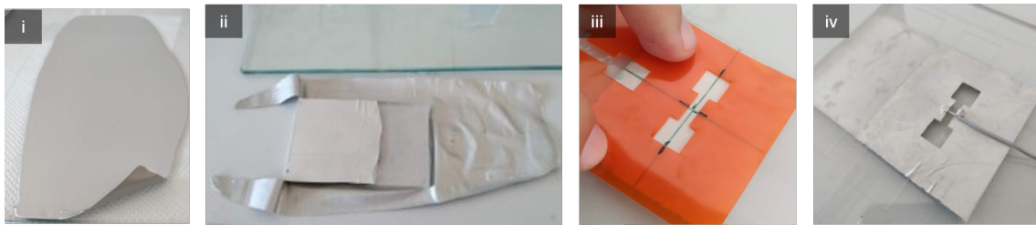
Figure 4.22: Stretchable proposed PIFA fabrication process. i: The stretchable conductive ink film is peeled of the glass, ii: then is folded over the substrate, and the excess is removed. iii: A previously cut stencil is placed on the top plane, and the aperture is cut with an x-acto knife. iv: The coaxial cable terminals are then connected to the film with small drops of the conductive ink.
