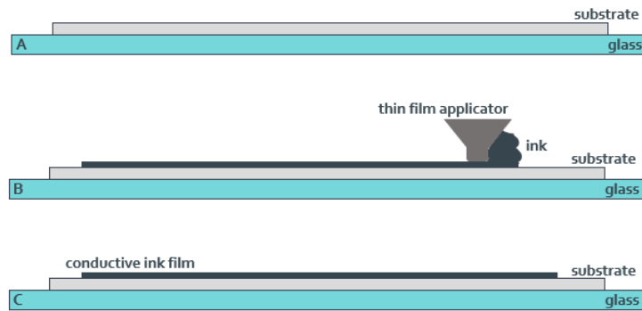
Figure 4.21: Schematic of the stretchable conductive layer fabrication process. A: The SIS layer is cured on top of a glass in order to cure uniformly. B: Ink is poured over the substrate and spread using a thin film applicator to ensure layer height. C: The ink is cured to form the conductive film.
