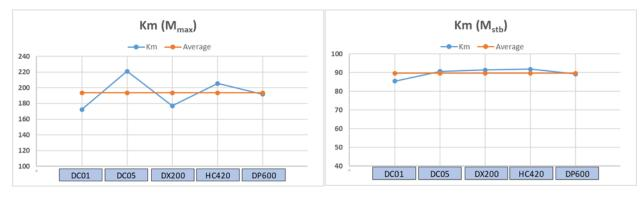
Figure 4.11 - Km values for maximum and stabilized torque
