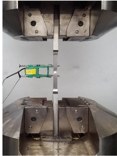
Fig. 3.4. Extensometer used for material characterization
