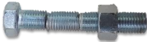
Fig. 3.25. Bolt failure – Group B: impact
