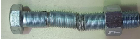
Fig. 3.18. Bolt shearing: Quasi-static test Group B
