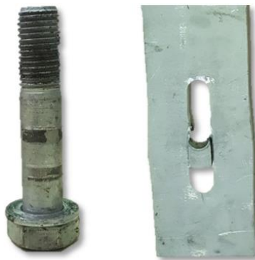
Fig. 3.27. Bolt and stainless steel plate after the tests: T5-M1-SI-10
