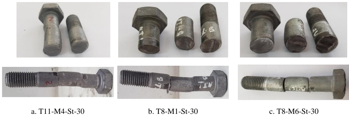
Fig. 3.16. Bolts after failure – Quasi-static tests Group A
