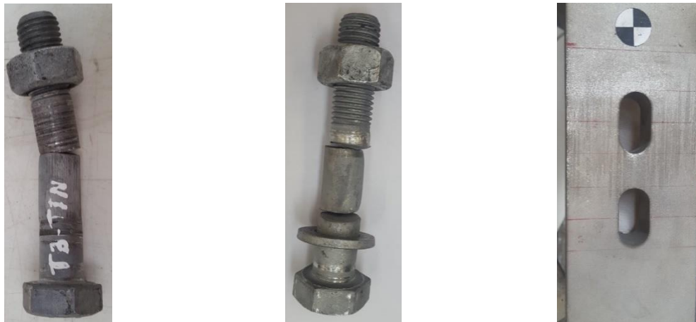
Fig. 3.23. Bolt and stainless steel plate after the tests- Group A, specimens with coating material M1
