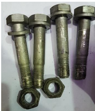
a. M16 bolts: nut stripping failure
