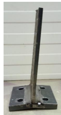
b. T-stub: deformation
