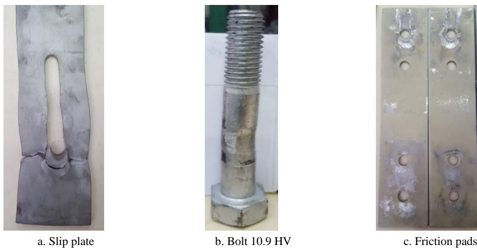
Fig. 3.21. Plates and bolt after the test - Quasi-static test Group C
