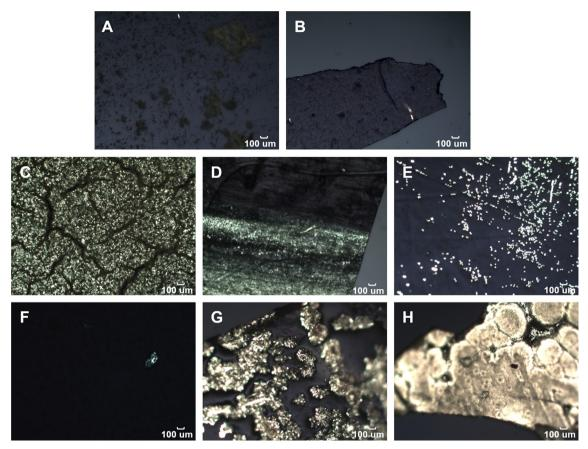
Fig. 4. POM images obtained with crossed polarizers for CSA as received (A); CSA film (B); and CA:CSA(X) electrolytes with X = 15.2 (C); 29.2 (D); 43.6 (E); 60.8 (F); 75.6 (G) and 82.3 (H).
