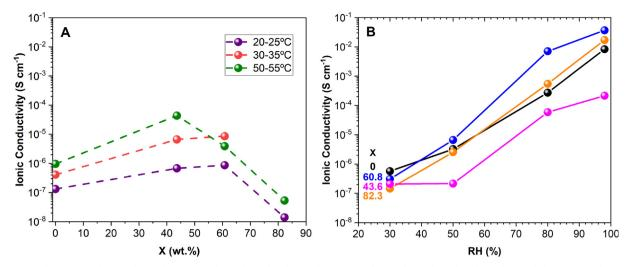
**Fig. 9.** Ionic conductivity isotherms obtained (A) at a relative humidity lower than 30% and (B) relative humidity dependence of the ionic conductivity under different RH at 25 °C for CSA and CA:CSA(X), with X = 0, 43.6, 60.8 and 82.3.
