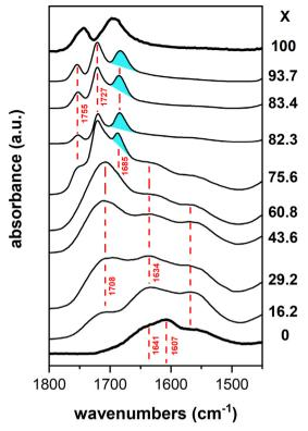
Fig. 3. ATR-FTIR spectra of CSA, CA and selected CA:CSA(X) electrolytes in the  $1800-1450 \text{ cm}^{-1}$  region. Blue shaded bands indicate the presence of CA monohydrate.
