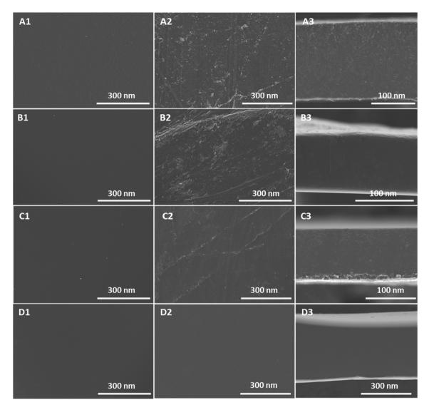
Fig. 5. SEM images of the top (1) and bottom (2) surface, and cryogenic temperature cross-section (3) of the CA:CSA(X) films, with X = (A) 15.2; (B) 29.2; (C) 43.6; and (D) 60.8.
