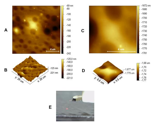
Fig. 7. AFM characterization of the CA:CSA(60.8) film: (A,C), 2D topographical and (B,D) 3D topographical images of 20 µm and 6.8 µm, respectively, obtained in resonant mode. (E) Image acquired on the AFM support prior to performing the analysis.
