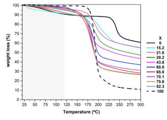
Fig. 8. TGA curves for CA, CSA and CA:CSA(X) electrolytes with X  $\,<\,$  83.4 in the 30–300  $^\circ C$  range.
