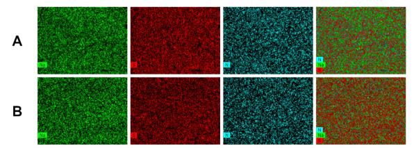
Fig. 6. EDS mapping images for the top surfaces of the CA:CSA(X) films, with X = 43.6 (A); 60.8 (B) for the elements Na (green), S (red) and N (cyan). The last column is a composite image obtained from the juxtaposition of all three elements.
