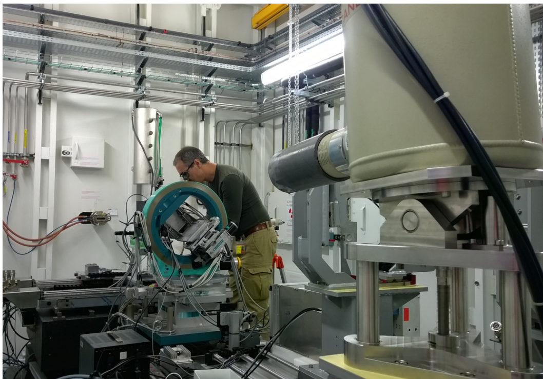
Figure 4.13: Opposite view of the beam pointing direction. It shows the beam entrance, the Compton-POLCA mounted to the 5-axis motorized stage and the Ge detector in the end of the line.
