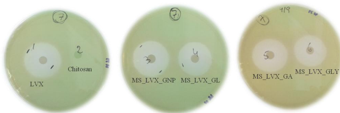
Figure 4.7 – Inhibition zones for LVX, chitosan and loaded MS crosslinked with GL, GNP, GA and GLY, for the bacterial isolates CF2_2004 (A) and CF7_2005 (B).
