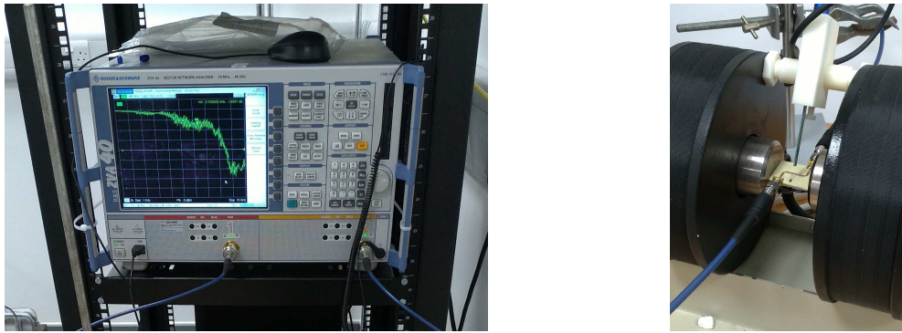
Figure 4.2: Picture of instruments used in room temperature setup: (left) VNA and (right) electromagnet with hall probe.
