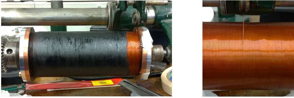
Figure 5.4: (Left) Finished solenoid mounted on the winding machine with final layer of stycast applied. (Right) Close up of the superconducting NbTi wire during the winding process.
