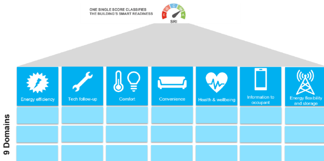
Figure 3.9. Calculation of SRI based on the equal weighting of seven impact criteria [26]
