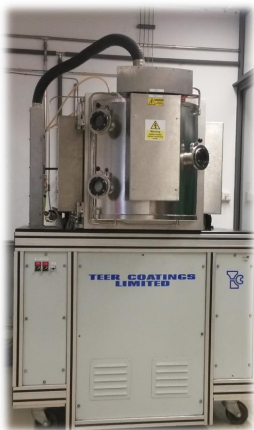
Figure 2.4 Magnetron sputtering equipment used in this work for deposition of WS-CF coatings.
