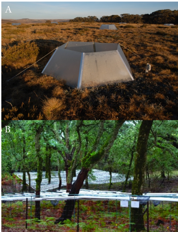
Figure 4: A: Example of open top chamber (OTC) (Wahren, 2019) B: Rain exclusion setup in Los Alcornacales (Jiménez et al 2018)
