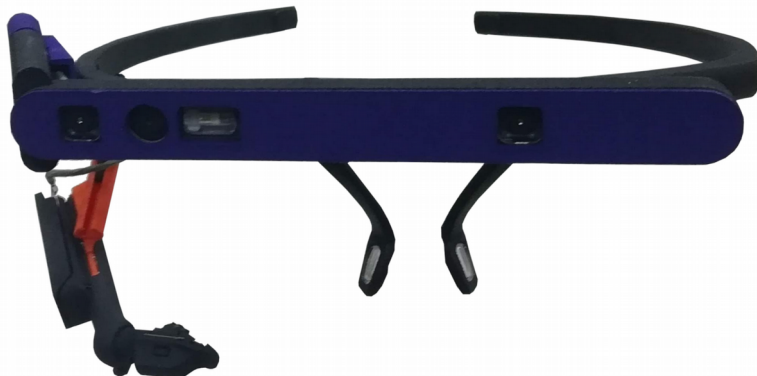
Figure 2: Photo of the Pupil Labs Eye Tracker used in the present dissertation, monocular version with the Intel Realsense R200 World Camera.
