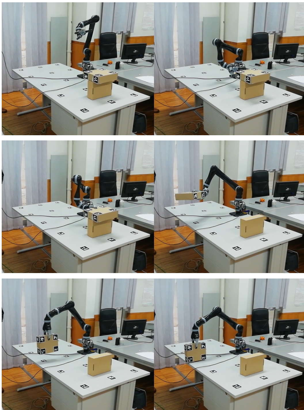
Figure 39: Video frames of the Pick and Place demo manual telemanipulation.
