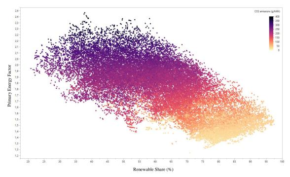
Figure 6.5. Relation between of primary energy factor, renewable share and CO<sub>2</sub> emission factor for 2014.
