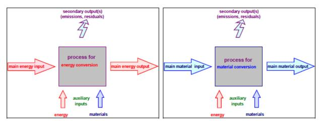
Figure 2.2- Unit processes for energy and materials conversion.
