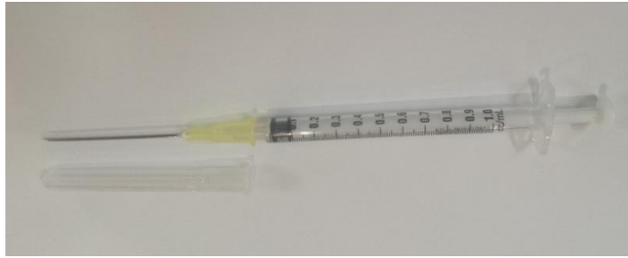
Figure 16 – Needle and syringe used as electrodes for CAP ejection.
