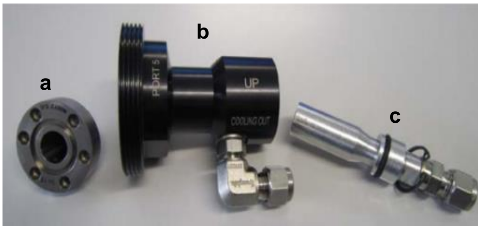
Figure 5 - Components of the niobium liquid target: a) conical target, b) target support and c) target diffuser. Adapted from (9).
