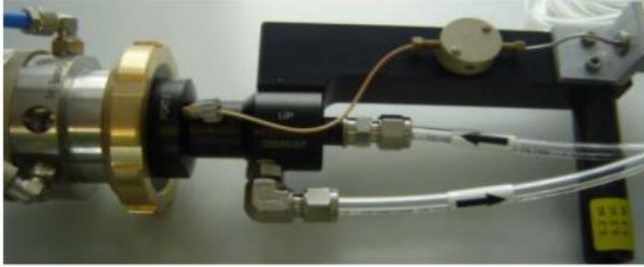
Figure 4 - Representative figure of the liquid target system. The arrows represent the water inlet and outlet. Adapted from (9).
