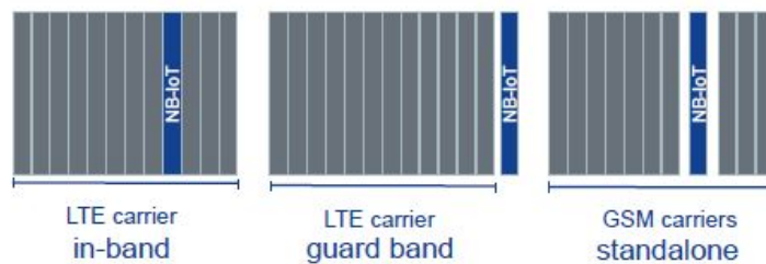
Figure 2.2: Configurable modes for NB-IoT deployment [13]
