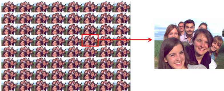
Figure 2.2: Sub-aperture representation of a Light Field.
