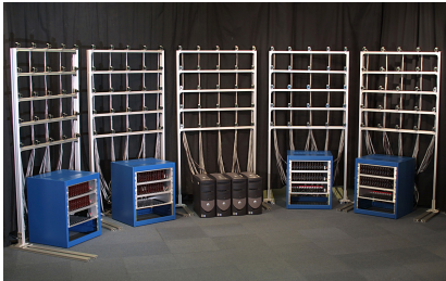
(a) The Stanford cameras array setup [14].
