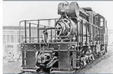
This ALCO 8-cylinder, 600 horsepower engine was typical of the engines being supercharged by Brown Boveri in the late 1920s (here with a VTx 300).
