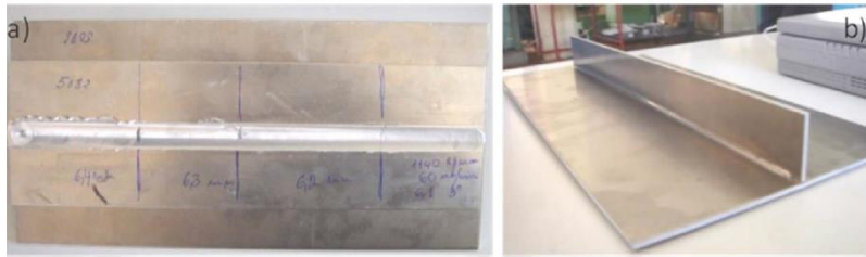
Fig. 5. Macrograph of a weld LP5-1. a) Skin side; b) Fillet side.
