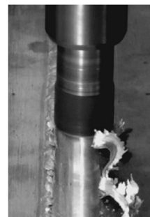
Fig. 2. Friction stir post-processing of a MIG_R plate.
