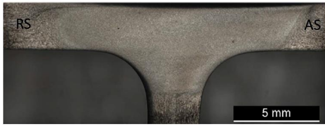
Fig. 12. Morphology of the 6082-T6 T-butt weld for specimen BPP6-1. RS-retreating side, AS-advancing side.
