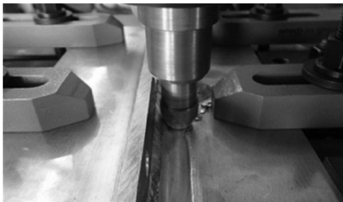
Fig. 2. FS processing of the GMAW T-fillet welds.
