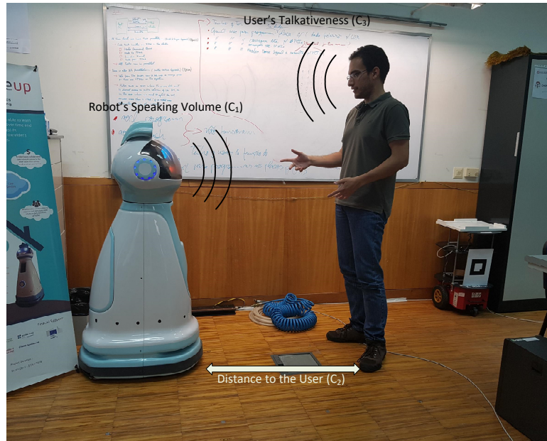
Figure 3.6: A picture of the experimental setup used for data gathering. The user faced the robot, speaking naturally while answering the robot’s questions. This allowed for the collection of all necessary measurements, as represented.
