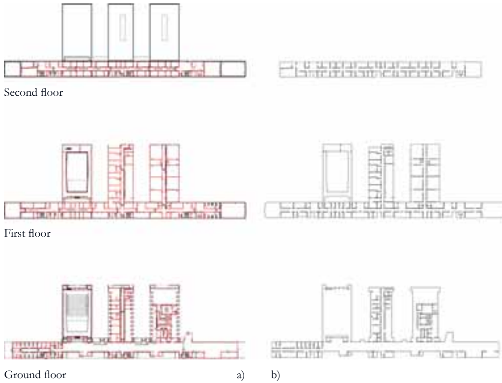
Fig. 176. Quinta das Flores School's new building: a) Closed polygons for axial maps over the final plans of the building (in red); b) Closed polygons for axial maps (Original plans provided by Parque Escolar, editing and closed polygons' drawings by Carolina Coelho)
