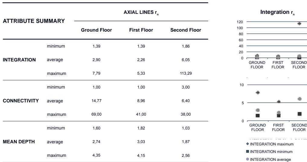
Fig. 181. Integration, Connectivity and Mean Depth r_n comparison for the axial line analysis (table and scattergram with and without outliers) (Carolina Coelho)
