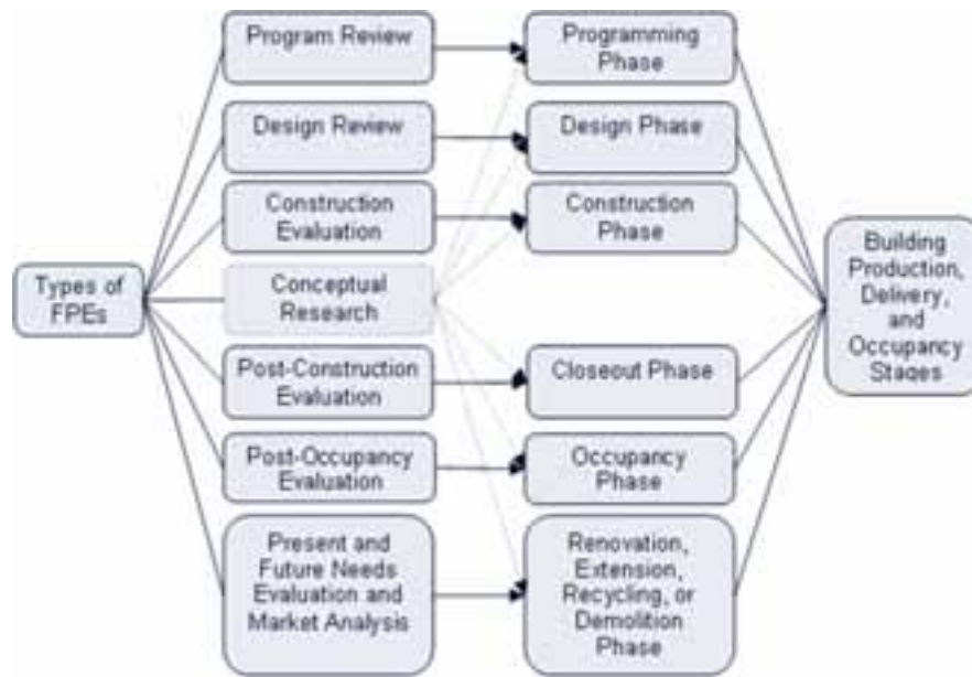
Fig. 88. “Types of FPEs and their relationships to the building production, delivery, and occupancy stages” (Zimring, Rashid and Kampschroer, 2005, p.2)
