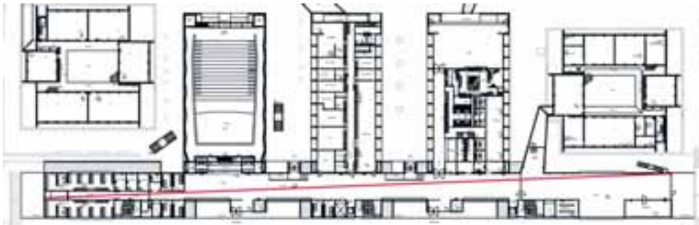
Fig. 137. Floor plan of Quinta das Flores School with its several convex spaces and a representative axial line (in red) (Carolina Coelho)
