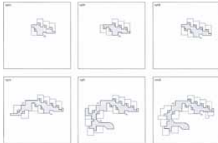
Fig. 59. Montessori School, Delft, by Herman Hertzberger, 1960-2010, plans of construction stages (Hertzberger, 2008, p.115)(Hertzberger, 2008, p.115; Hertzberger, 1991, p.29)
