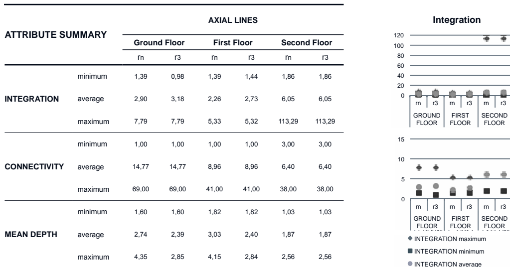
Fig. 182. Integration, Connectivity and Mean Depth r_n and r_3 comparison for the axial line analysis (table and scattergram with and without outliers) (Carolina Coelho)
