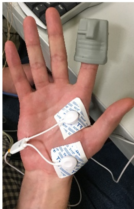
Figure 4.2: BiosignalsPlux's sensors (white) positioned for EDA measuring. The index finger's sensor measures PPG and is connected to the Sensatron equipment.
