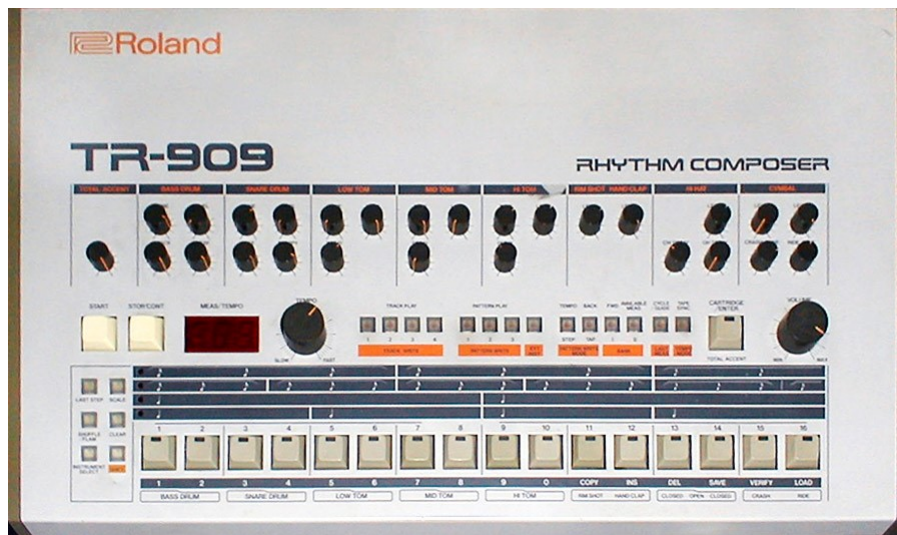
FIGURE 4.7: Roland TR-909 Rhythm Composer, a landmark tool in the genesis of house and techno music. Each of the 16 buttons at the bottom refer to a 16 th note or a step. Source: https://en.wikipedia.org/wiki/Roland_TR-909
