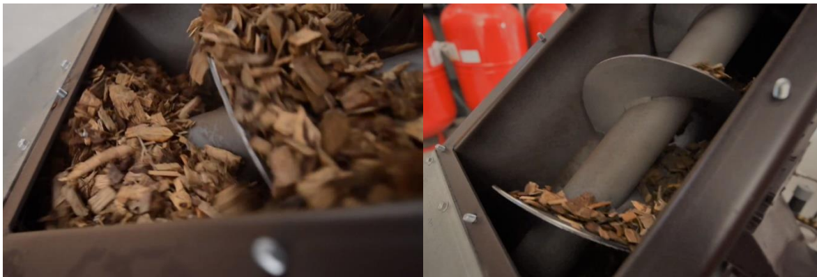
Figure 2.2. (a) Biomass carried by worm-screw (b) Worm-screw and structure.
