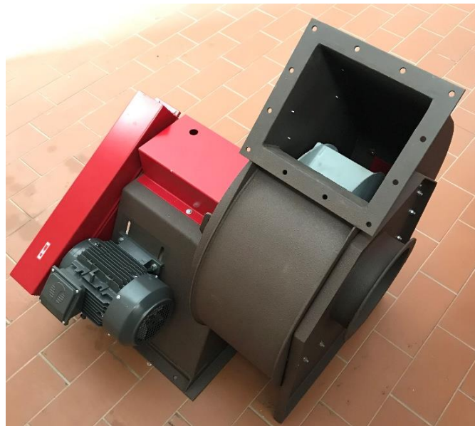
Figure 2.6. Induced draft fan for the boiler system.
