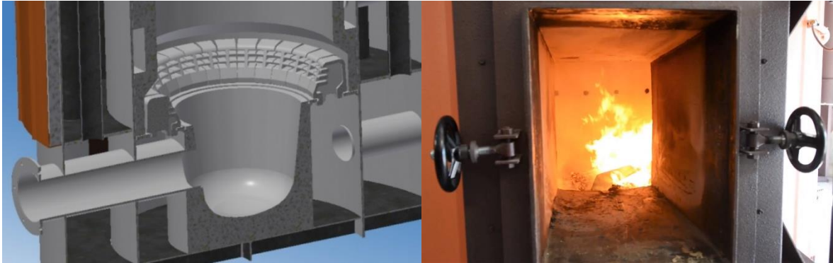
Figure 2.3. (a) CAD model of the chamber's lower section (b) Furnace door where biomass is transferred.
