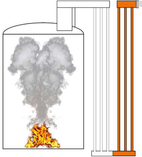
Figure 4.6. Total area of the 3 rd pass represented in orange, which considers the area of the two sets of smoke tubes, half of the second inversion box and the whole third inversion box (chimney).
