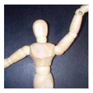
Figure 37: **Wooden dummy used as an imaging target**: the body of the dummy is made of wood, while an interior metallic wire allows member and torso flexibility.
