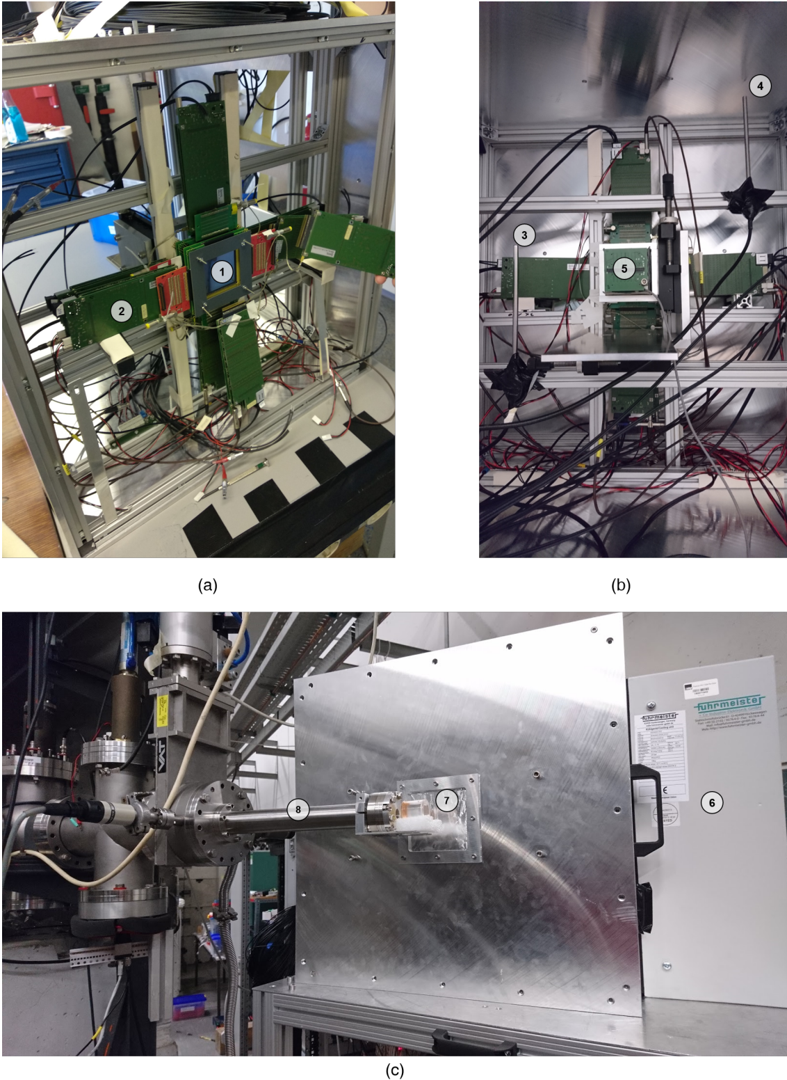
Figure 3.10: Photographs of the Compton camera mounted at a beamline of the Maier-Leibnitz-Laboratorium (MLL) in Garching during a beam time at the local Tandem accelerator. In a) the front view of the camera is presented, where the DSSSD detector (1) and its readout system (2) are visible, while in b) there is shown the back view from where the absorber component (5) and temperature sensors ((3) and (4)) are visible. In c) the closed Compton camera can be seen with the cooling system on the right side (6) and with the entrance window (7) as well as the beam line (8) with exit window flange and cylindrical water target in the front. 41
