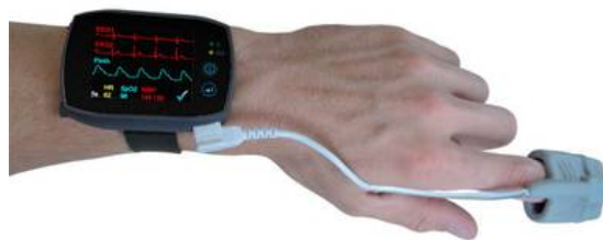
Figure 3.4: SOMNOmedics TM combines the pulse transit time with ECG and SpO2 finger clip to calculate blood pressure [8].
