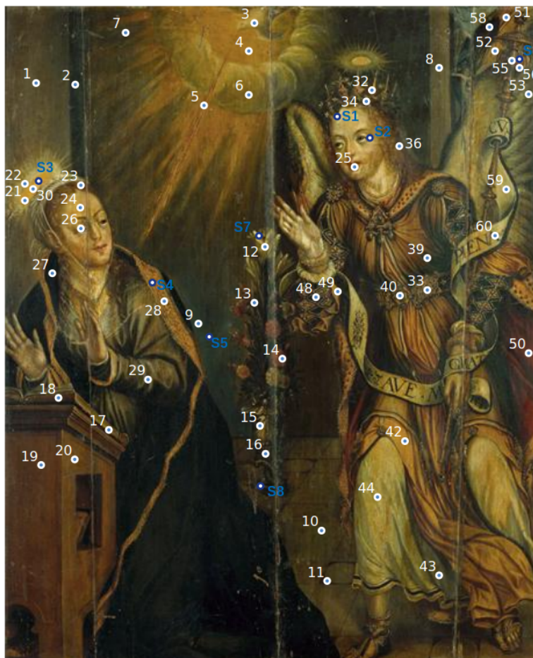
Figure 4.1: Samples obtained using PXRF, at white, and samples extracted, at blue, from the painting Annunciation (P25) . Original image provided by MNMC.
