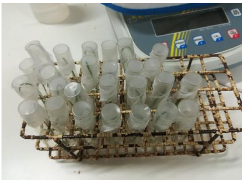
Figure 4 –Needles placed in test tubes with distilled water for SW measurements
