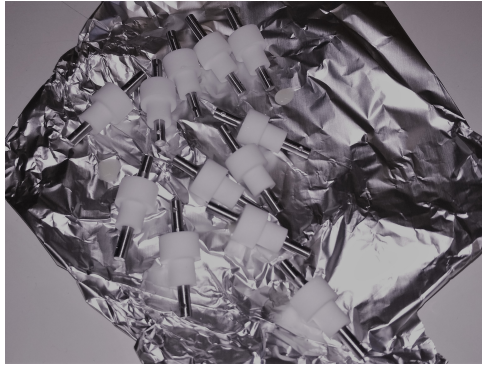
Figure 4.3: Photograph of the feedthroughs after the gluing process.
